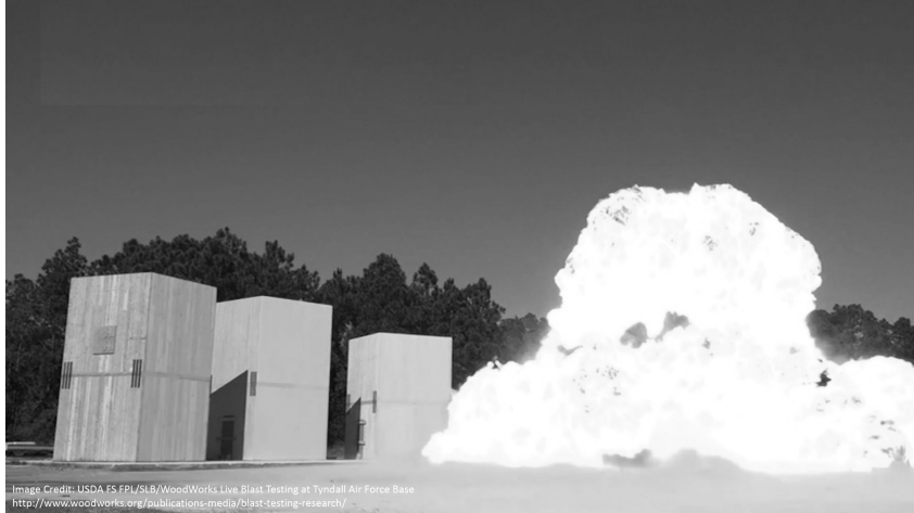
Image Credit: USDA FS FPL/SLB/WoodWorks Live Blast Testing at Tyn dall Air Force Base http://www.woodworks.org/publications-media/blast-testing-research/
